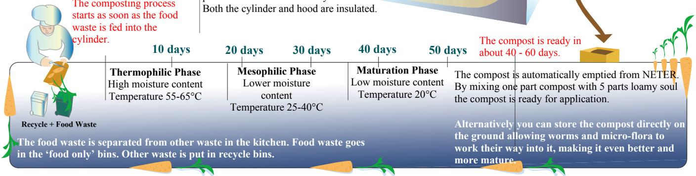
The compost is automatically emptied from NETER. By mixing one part compost with 5 parts loamy soil the compost is ready for application.
